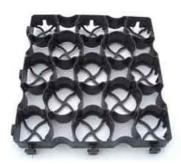
The tough, durable interlocking grid system is designed to provide ground reinforcement, turf protection and erosion control. Two verges which have been completely destroyed are to be evenly flattened, two to three inches of sand laid and the "grass road" embedded. Once settled, it will be filled with top soil and grass seed to allow grass to grow through. This will then stop the damage to the grass verges, provide sturdy ground for parking on and still allow for grass cutting to take place.
