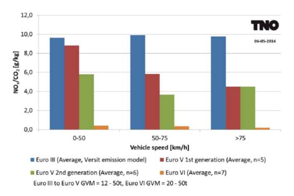
Figure 14: Trend of the average real-world NO<sub>x</sub> emissions of heavy-duty diesel vehicles from Euro III to Euro VI, over three different speed ranges. The Euro VI vehicles in this picture are the average of the vehicles tested. These vehicles have a Gross Vehicle Mass from 20 to 50 tonne, whereas the Euro III to Euro V have a GVM of 12 to 50t.
