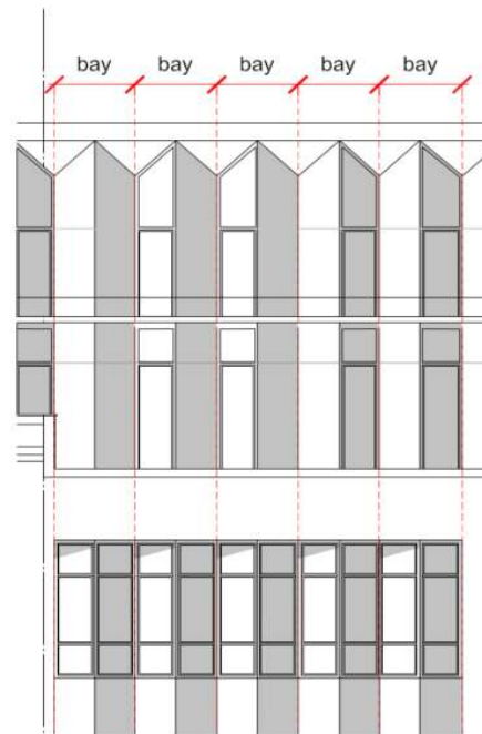
Proposed cladding aligned with existing below
