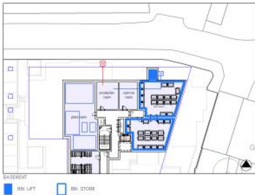
waste and recycling storage at basement level
