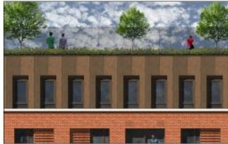
COPPER-BRONZE CLAD METAL CLERESTORY
