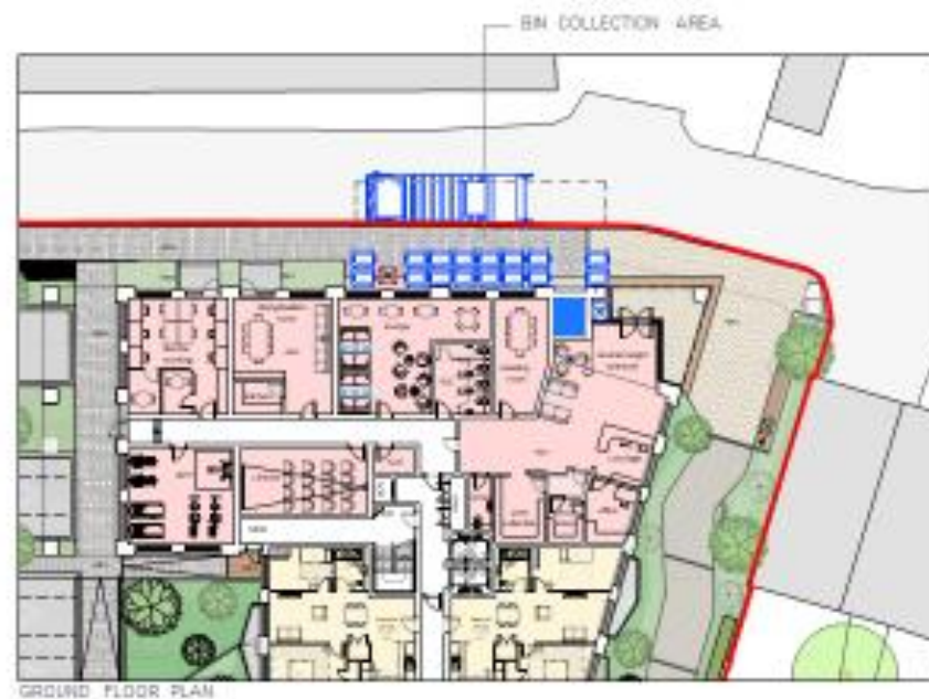
bins to street level via dedicated lift for collection
