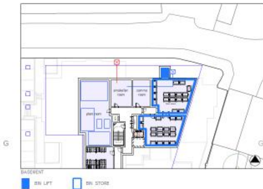
waste and recycling storage at basement level
