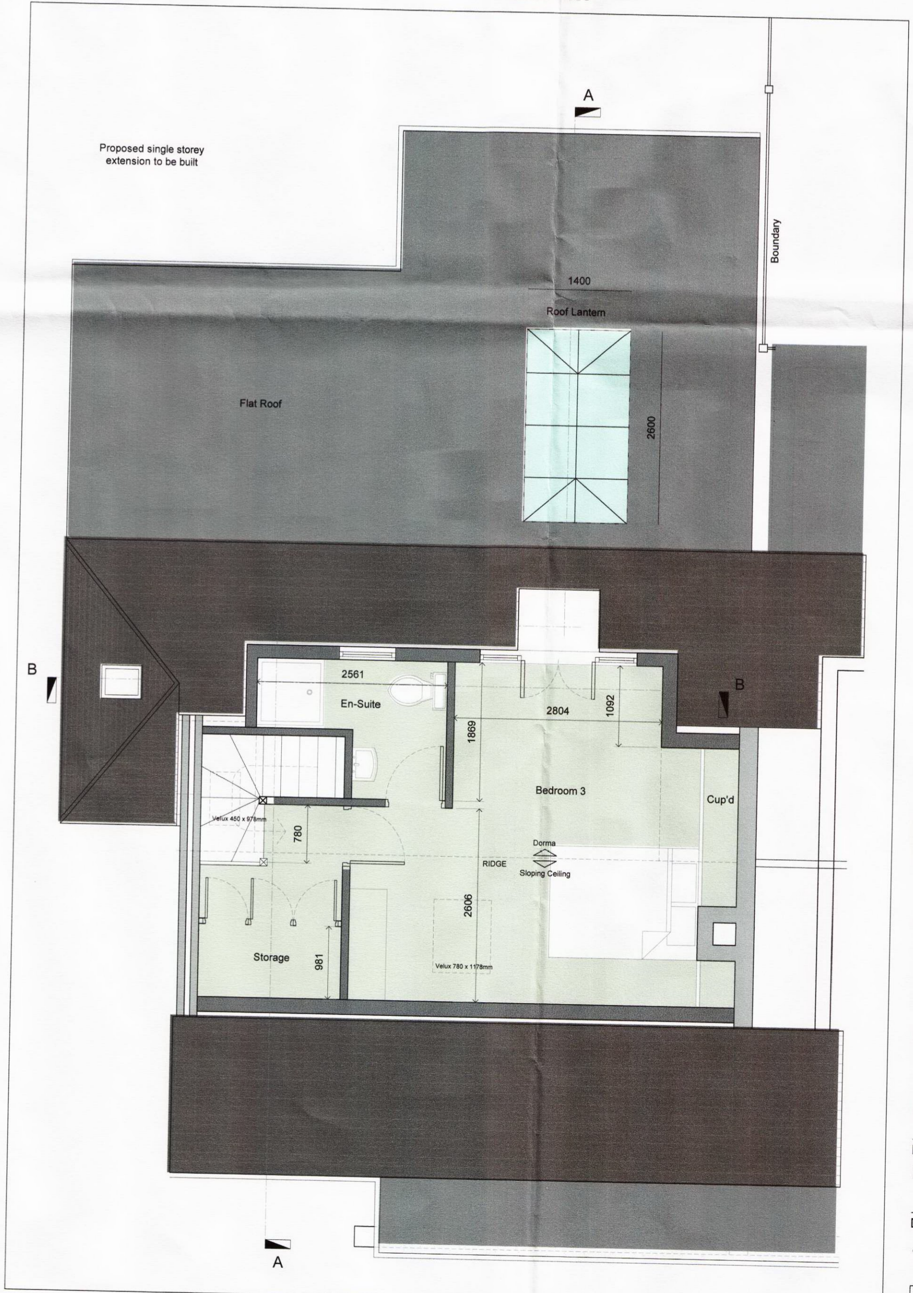
First Floor / Roof Plan
