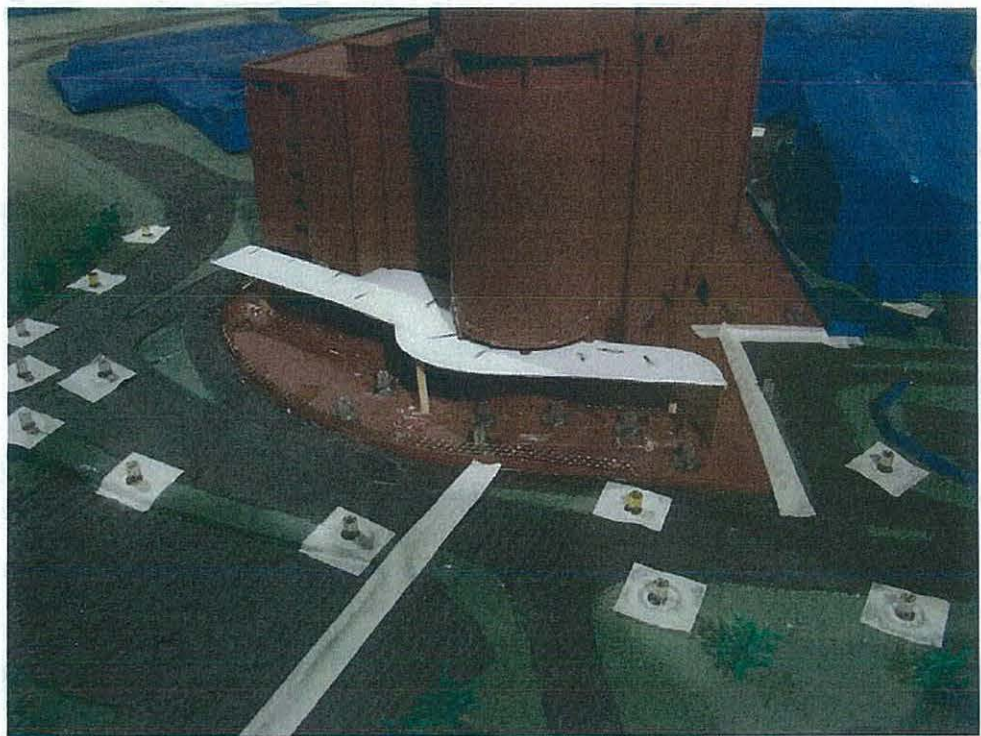
Figure 1d: Model as tested in wind tunnel – Configuration AF.
