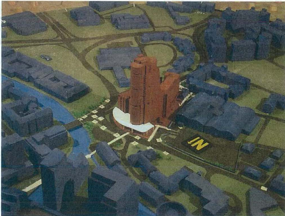
Figure 1b: Model as tested in wind tunnel – Configuration AD.
